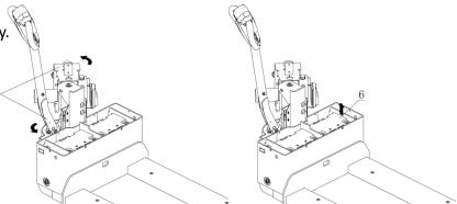
Install the battery in the reverse order to see if the battery is loaded and the wiring is correct. Put the battery cable in place to ensure that no shear occurs when placed in the battery.
