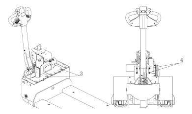
E: Rotate the handle to the extreme position of the diagram, then rotate the electrical panel as shown in the diagram until it is completely free of occlusion of the battery.
