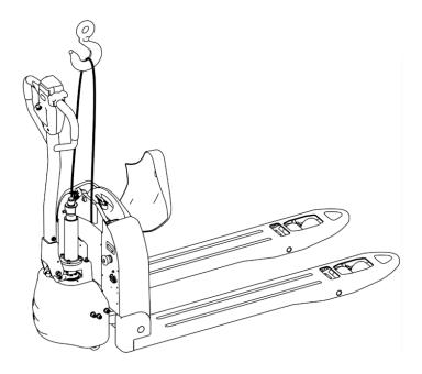
○,3 When moving the truck.Pay attention to keep the center of the moving truck in the middle of two fork
