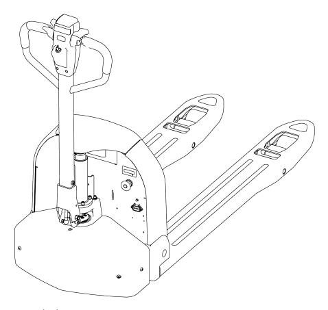
CBD15/18/20J-Li3 is a walkie electric pallet truck. It adopts the advanced structure such as ring rod lifting system and new ac controller, at same time it is equipped with high quality motor, lithium battery and pump station motor. It has the characteristics of superior performance, convenient operation, flexible steering, reliable braking, good dynamic performance, less noise, less pollution and beautiful appearance.
