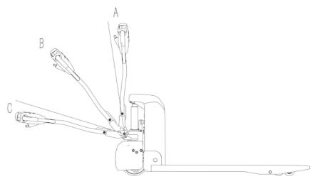
Slowly rotate the accelerator to start the truck. (In order to be safe, fast acceleration is prohibited.)
