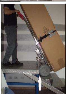
Only after the trolley has "hopped" can the two large grey wheels then be moved forward because the mechanism is ready to go down to the next step.
