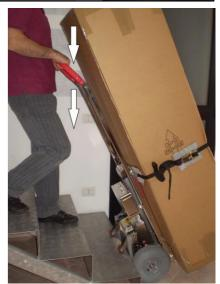
5. Once you have climbed the step, as soon as the two large grey wheels are resting on the step itself, pull them until they are resting completely against the next step (SEE THE RIGHT WAY AT POINT NO. 3) and start from this point.
