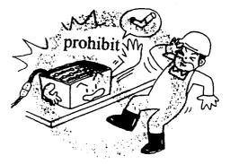
– Do not approach tools to the two poles of the battery, which can cause the sparkle.
