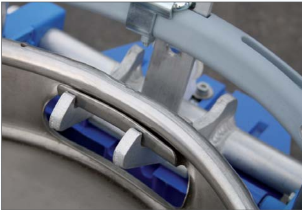
The height-adjustable hook permits KEG drums of various sizes to be transported, therefore simplifying the logistics of these cylindrical goods.
