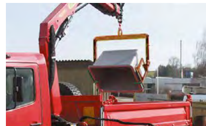
Tipping the grit out onto a truck platform (shown with 700 L the grit container)
