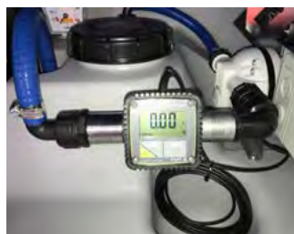
Meter FMT 3 with pulse output
