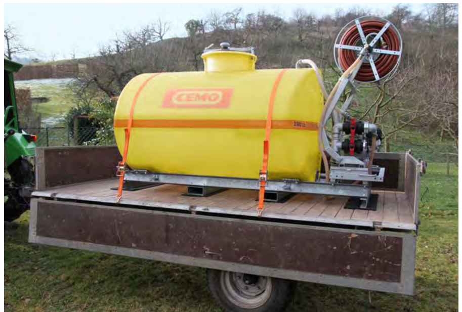
Securing loads with anti-slip mats and lashing straps (lashing down) using the example of a 2000-litre mobile irrigation system
