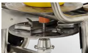
Stainless steel spreader disc, adjustable
