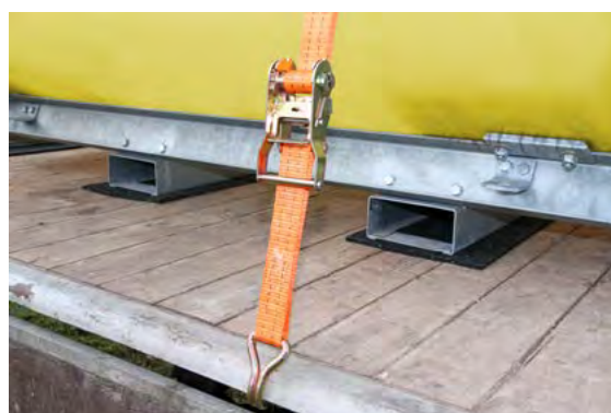
Securing loads with anti-slip mats and lashing straps (lashing down) using the example of a 2000-litre mobile irrigation system
