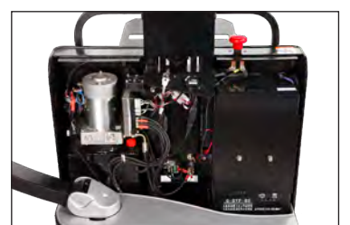
Built-in charger and maintenance free batteries
