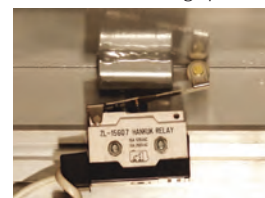
The upper platform has a safety frame that covers all four sides. There are double switches for lowering safety of the platform.
