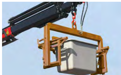
Lifting the container (shown with 200 L the grit bin)
